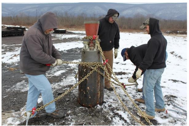
Crew members of Letterkenny Munitions Center prepare a rocket motor for open burning destruction. The rocket motor is chained down to ensure the safety of the employees and surrounding facilities. Depending on size, up to 20 can be treated at one time lasting several minutes.
